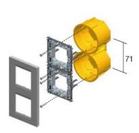
Frame mounts over wall box, screws allow alignment if required.
