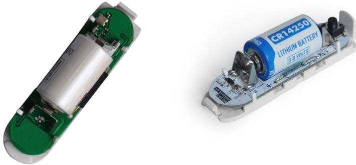
Disassemble the door sensor      Install battery, assemble the door main body .
