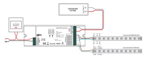
Note: only the RGB LED can be controlled under this mode.
